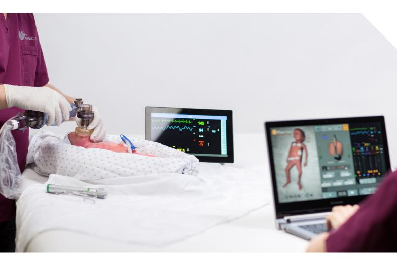
The entire system comprises the preterm baby simulator Paul, the management computer with control software and a patient monitor. Paul is controlled and operated without the need for any wires.
